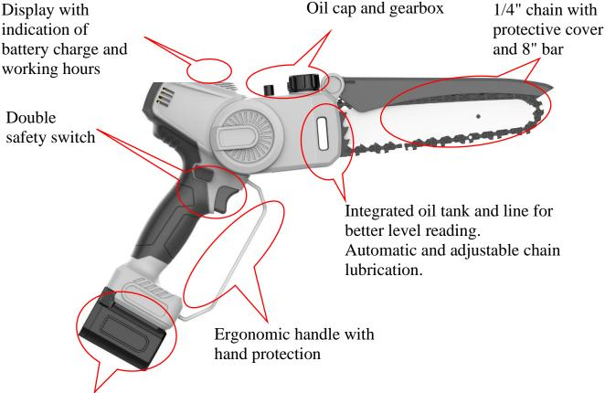
Quick-connection rechargeable lithium battery 21,6V 4Ah
