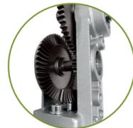
NUOVA TRASMISSIONE CON INGRANAGGI ELICOIDALI
