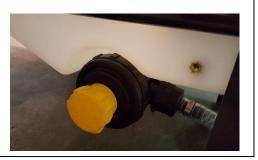
DRAINING CAP: UNSCREW THIS CAP TO WASH, CLEAN AND EMPTY THE WHEELBARROW FROM REMAINS OF PRODUCT. THEN CLOSE THE CAP VERY WELL IN ORDER TO AVOID LEACKAGE OF PRODUCT.
