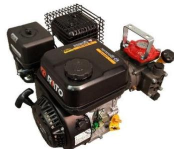
**MOTO/ELETTRICO POMPA:** LA MOTO/ELETTRICO POMPA CONSTA DI UN MOTORE A SCOPPIO 4 TEMPI BENZINA OPPURE DI UN MOTORE ELETTRICO MONOFASE, QUESTI SONO COLLEGATI TRAMITE RIDUTTORE DI GIRI AD UNA POMPA A MEMBRANA MARCA ANNOVI E REVERBERI AR202 OPPURE AR252.
